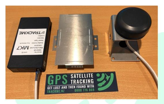
Device with cable attached to External Aerial and alongside Alloy casing for protection and mounting.
