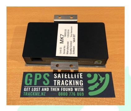
Side entry power cable shown allows for secure connection and no loss of data from unsecured connections. Right angle power connection supplied.
